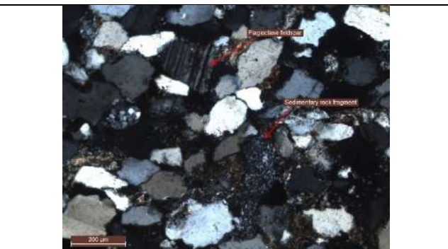
Figure 2: Photomicrograph showing Plagioclase Feldspar, and Sedimentary Rock Fragment
