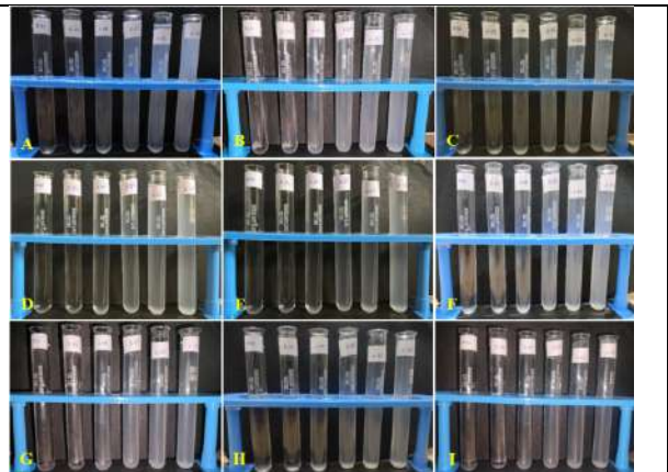
Figure 7: Silica Nanoparticle Suspension in Nanofluids in 0 Hour (A), 12 Hour (B), 1 Day (C), 2 Day (D), 3 Day (E), 4 Day (F), 6 Day (G), 8 Day (H), and 10 Day (I).
