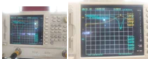
Figure 5. (a) Measured result of proposed reconfigurable Band Pass Filter for case 1 (b) Measurement using VNA for case 2 (Agilent 8722ES 50MHz-40GHz).
