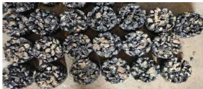
Figure 1 OGFC samples with different compaction efforts
