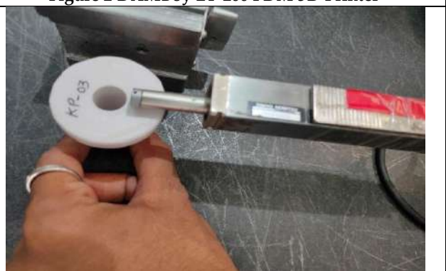
Fig.4 Mitutoyo SJ-210 surface roughness tester
