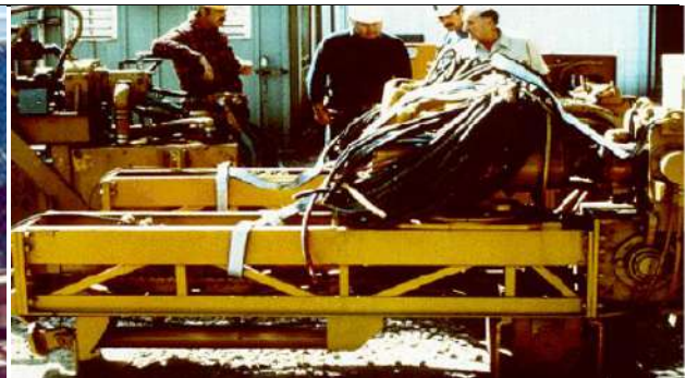
Fig. 4. (c) Small Frame-Mounted Rotary Hydraulic Drill Rig
