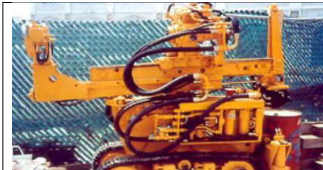
Fig. 4. (b) Low Headroom Track-Mounted Rotary Hydraulic Drill Rig
