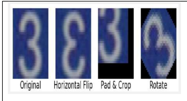
Fig 1 : An image of the number "3" in original form and with basic augmentations applied.
