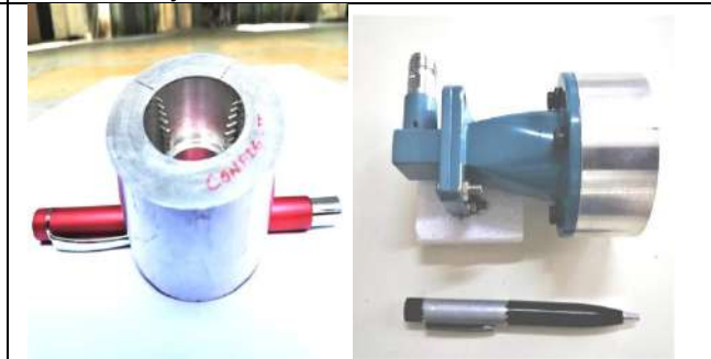
Fig. 6. Images of fabricated dual mode horn with and without rectangular to circular transition.
