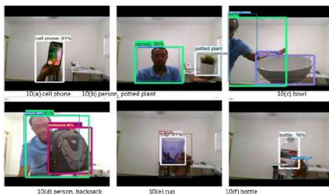
Figure 9: Positive prediction on a trained objects based on RetinaNet Algorithm has examined in 9(a) as cell phone with 91%. 9(b) the object person has identified with 100%. 9(c) the object chair has identified with 69%. 9(d) the objects person and backpack has identified with 86% & 95%. 9(e) the object cup has identified with 23%. 9(f) the object bottle has identified with 76% accuracy and wrong predictions as chair and person with 99% & 99%.
