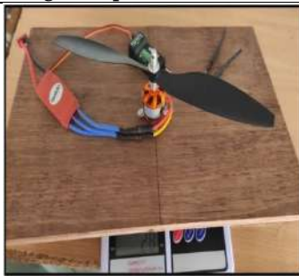
Fig 7. Thrust testrig to identify the motor thrust
