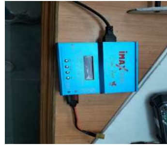
Fig 6. LiPO battery charger for drones
