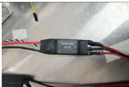
Fig 2. ESC brushless motor controller
