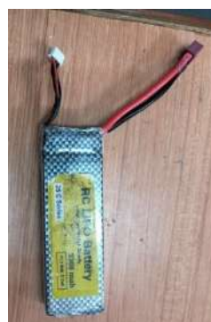
Fig 4. LiPO Battery for RC crafts and drones
