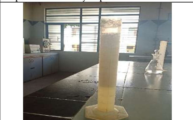
Figure 6: Foam height of F4 after shaking
