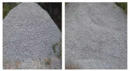
Fig 2 :20mm and 12mm Coarse Aggregates
