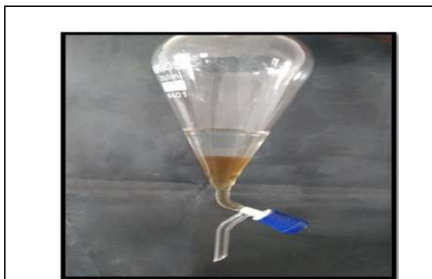
Fig 1: Diethyl ether extraction of ellagic acid using separating funnel
