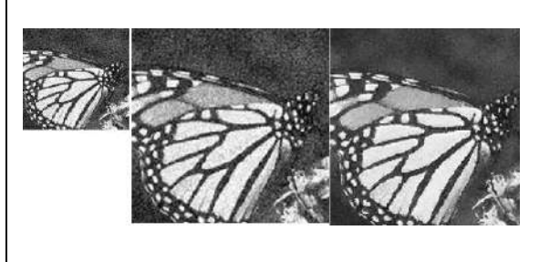
Figure 3: (a) Low resolution image with Gaussian noise ( \sigma=0.2 ) (b) Cubic spline interpolated image (c) Super resolved images
