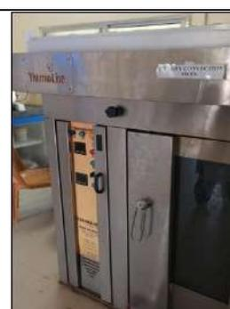
**Fig.2. Rotary convection oven**
