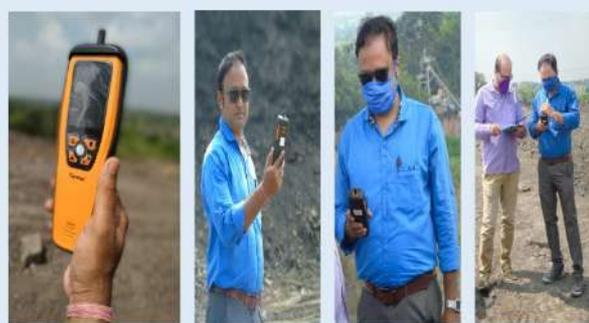
Figure 4. Air quality of Kalipahari OCP patch-A, Kalipahari colliery was measured at different spots through Temtop M2000C Air Quality Monitor
