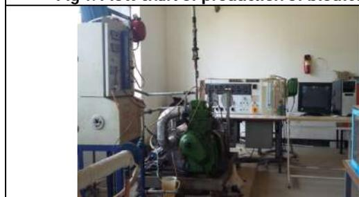
**Fig 3: CI engine test rig**
