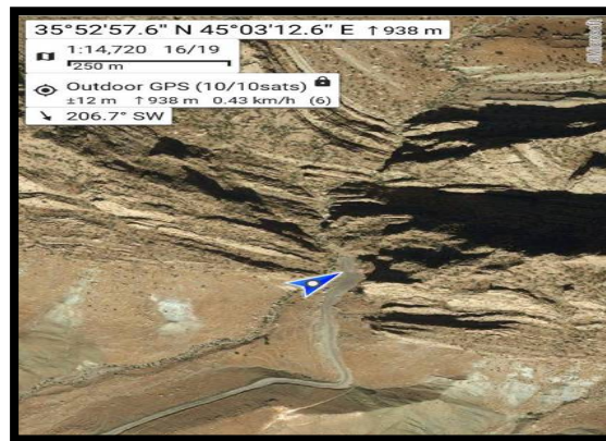
Figure 16. Satallite image shows the dextral strike-slip fault in Jasana gorge
