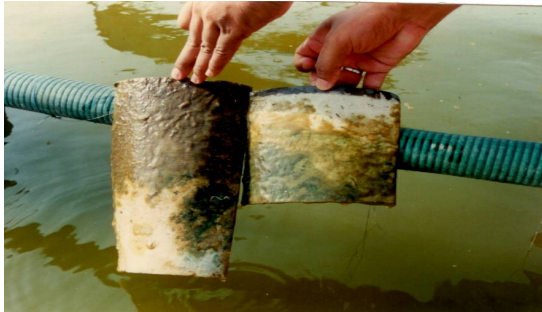
Fig. 1. Long plate not coated with commercial grade synthetic enamel paint. Small plate coated with OHUCAX additive. Margins of small plate left bare.
