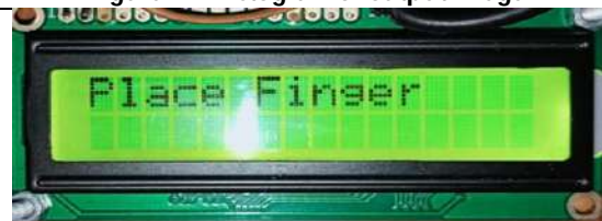
Figure 13: Output of fingerprint sensor.
