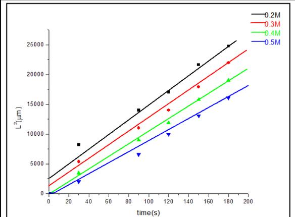
Fig.10 Plot of L<sup>2</sup> vs time for different concentration of AOT
