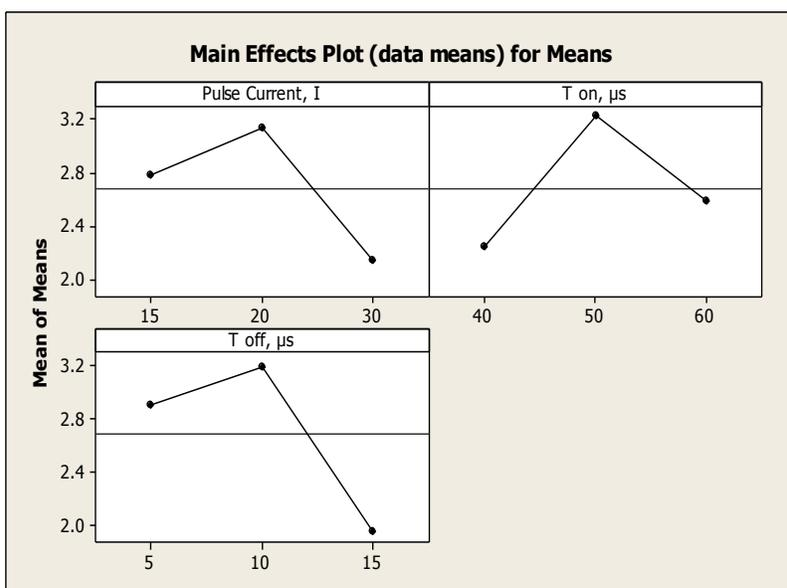
Fig. 2. Main Effect Plot (Copper Electrode)
