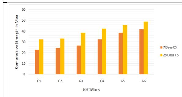
Fig. 1: Compressive strength of GPC in 7 and 28 days
