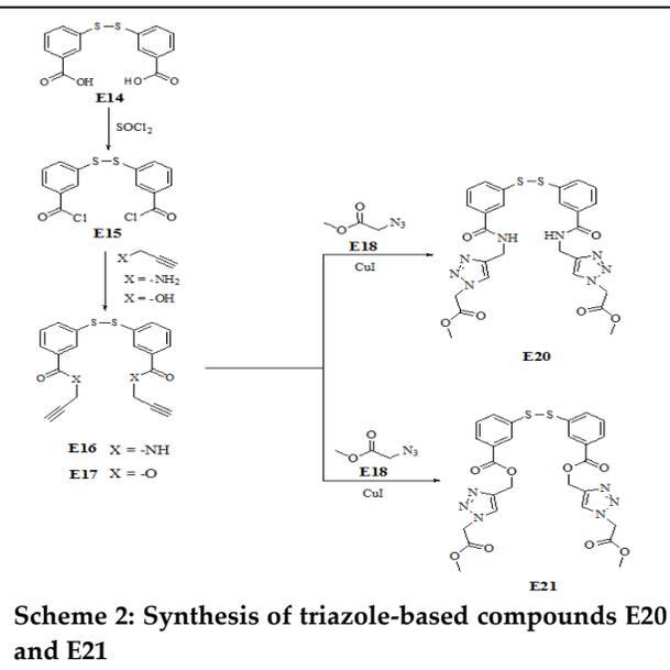
Scheme 2: Synthesis of triazole-based compounds E20 and E21
