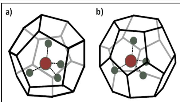
Figure3: Methane hydrate structure: the rigid cages are composed of hydrogen-bonded water molecules, and each cage contains a methane molecule. Source, courtesy of the Mount Elbert gas hydrate stratigraphic test well project
