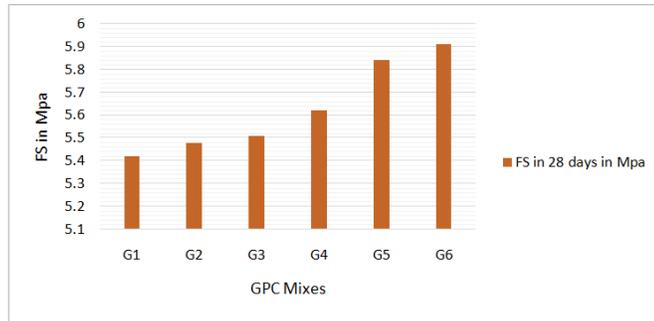
Fig. 3: Flexural strength of GPC in 28 days
