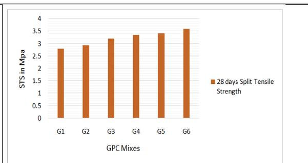
Fig. 2: Split tensile strength of GPC in 28 days
