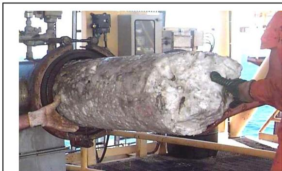
Figure 5: Specimen of methane hydrate extraction, source: courtesy of the NGHP-1, India
