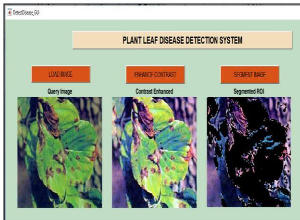
Figure 8: Image Pre-processing using Color Transformations and Masking Green Pixels
