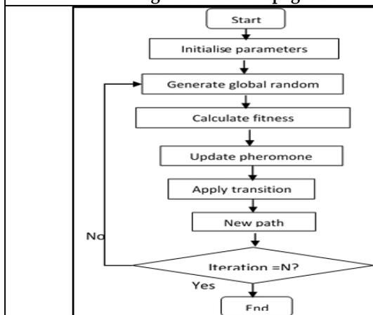
**Figure 3: Flow Chart of Ant Colony System**
