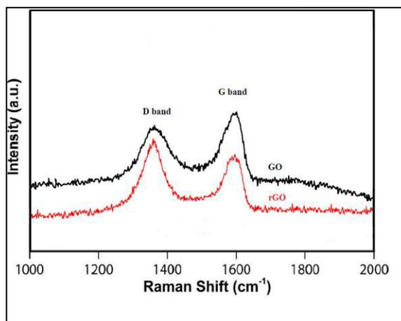
Figure. 5. Raman Spectra of GO and rGO
