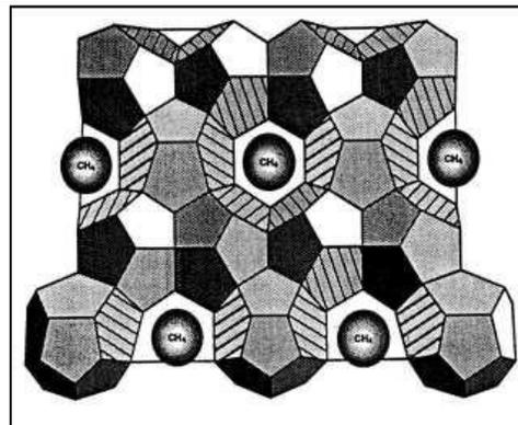
Figure2: Water molecules are arranged in a rigid frame work of cages, Source, courtesy Krason and Ciesnik1985
