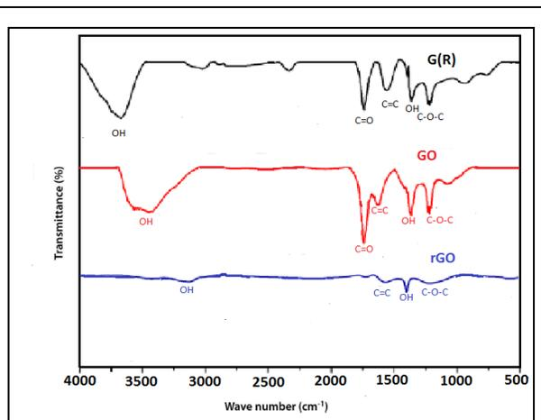
Figure.3: FTIR Spectra of G(R),GO and rGO
