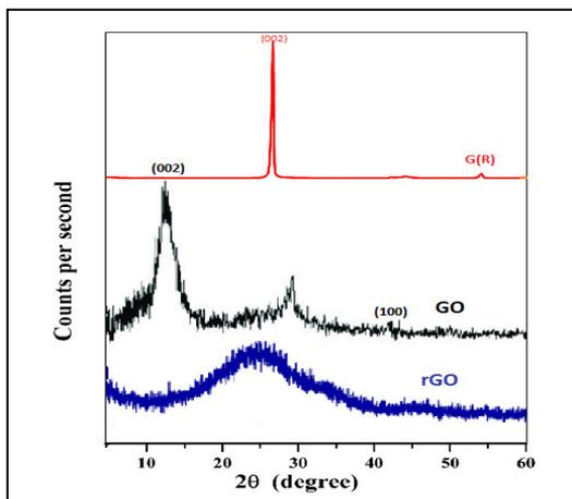
Figure. 4. XRD Pattern of G(R),GO and rGO
