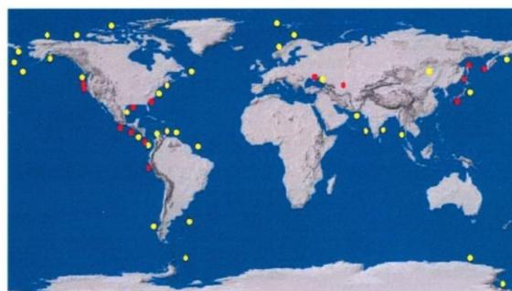
Figure4: Location of gas hydrates in oceanic sediments along continental margins and in polar continental settings. Source: Loreson TD and Kvenvoloden KA: *A global inventory of natural gas hydrates occurrence*, USGS, <http://walrus.wr.usgs.gov/globalhydrate/index.html>
