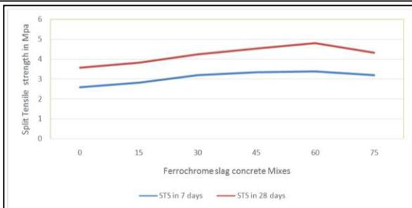
**Fig. 5: Split tensile strength in Mpa**
