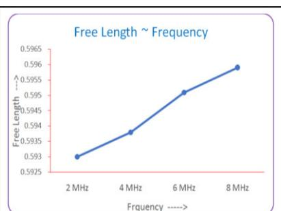
**Fig. 2: Variation of free length with frequency**
