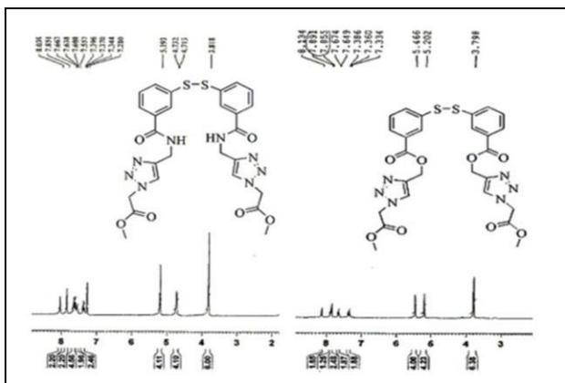
Figure 3: <sup>1</sup>H NMR Data of E20 and E21 to compare the range from 3-6 ppm for di-triazole product formation
