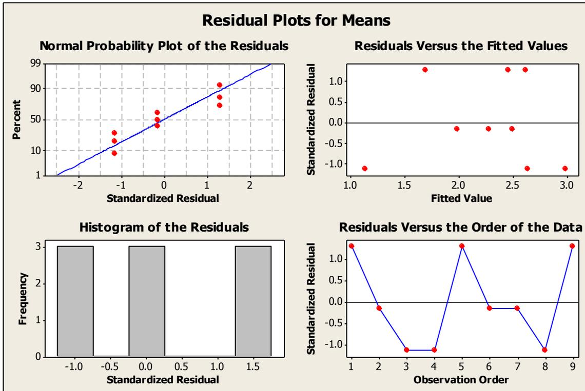
Fig .3.Residual plots (Brass Electrode)
