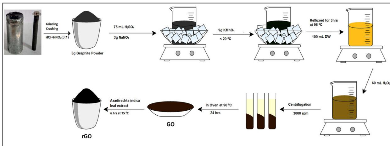
Figure. 1. Systematic procedure of synthesis of GO and rGO from graphite powder obtained from waste battery cells.
