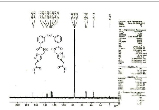
Figure 6: <sup>13</sup>C NMR (75 MHz, DMSO-*d*<sub>6</sub>) spectrum of compound E20
