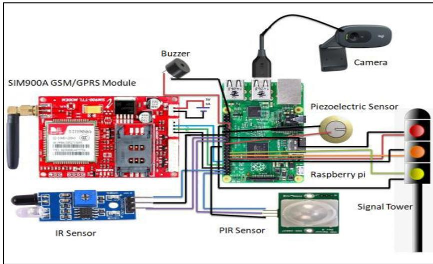
Fig. 2: Circuitry Diagram of whole Hardware Structures
