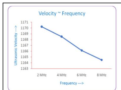
**Fig. 1: Variation of ultrasonic velocity with frequency.**
