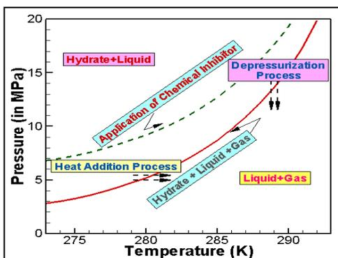
Figure: 7 Decomposition of hydrates by depressurization, thermal, and chemical techniques e.g., Hunt, 197; source R.C. Selly
