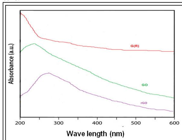
Figure.2. UV-Vis spectra of G(R),GO and rGO.
