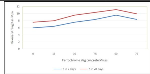
**Fig. 6: Flexural strength in 7 and 28 days in Mpa**
