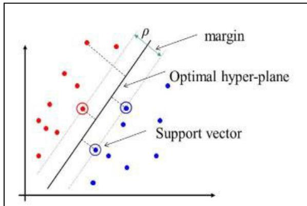
Figure 4: Optimal Hyper Plane separating Support Vectors in SVM
