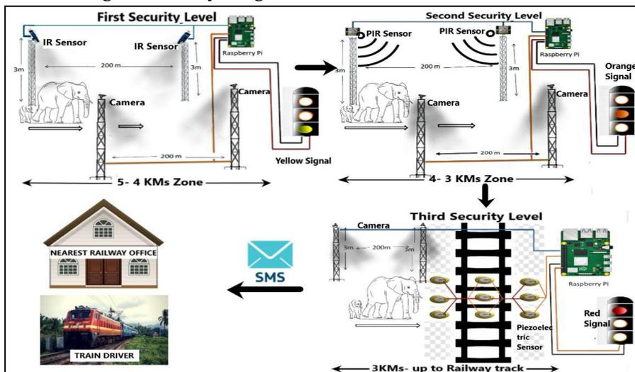
Fig. 3: Three Security Layers ranging from 5KMs up to railway track in Elephant trespassing zone
