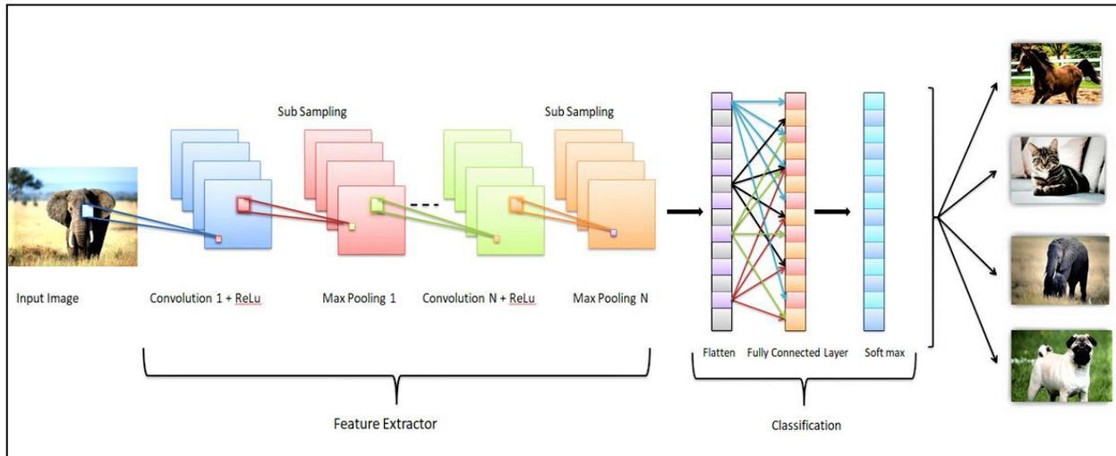
Fig. 4: Phases of Classification using Convolution Neural Network
