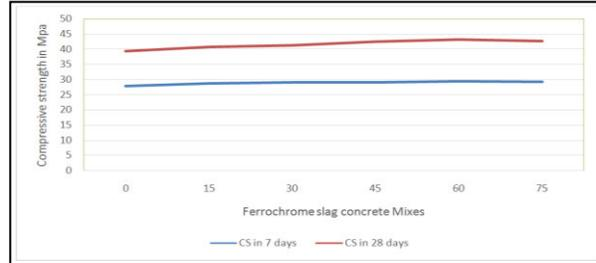
**Fig. 4: Compressive strength of ferrochrome slag concrete in 7 and 28 days**
