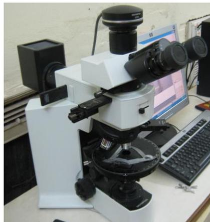
Fig.2 Olympus BX51 Optical microscope
