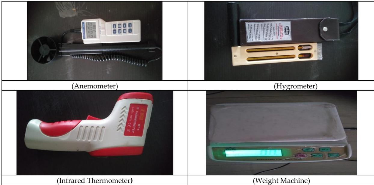
Figures 2 showing various types of measuring instruments during testing and analysis
