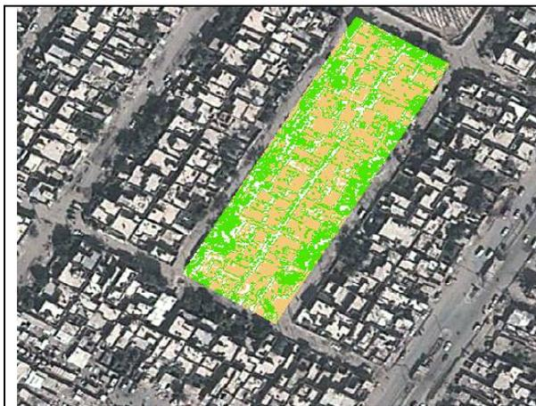
Figure (7-a): The resulted three classes' raster after the application of classification technique of the resulted raster from the collection process of typical part of Hey Ur scene.
